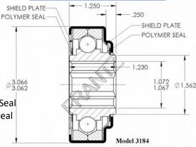
\* Also press fit into 3-1/4" x 13g, 3-1/4" x 12g, 3-1/2" x 7/32", 3-5/8" x 9/32" and 3-3/4" x 11/32" tubes.
